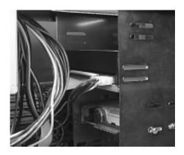
Audio Cable (optional) - If you have a sound card and speakers, and would like to play audio CDs on your computer, you will need to get a sound cable. Contact AMC, our small parts supplier, at 888/262-9700. Sound cables are made for the sound card you are using and the DVD-ROM to which you are connecting. Make sure you have this information when purchasing a sound cable. The sound cable connects to your sound
